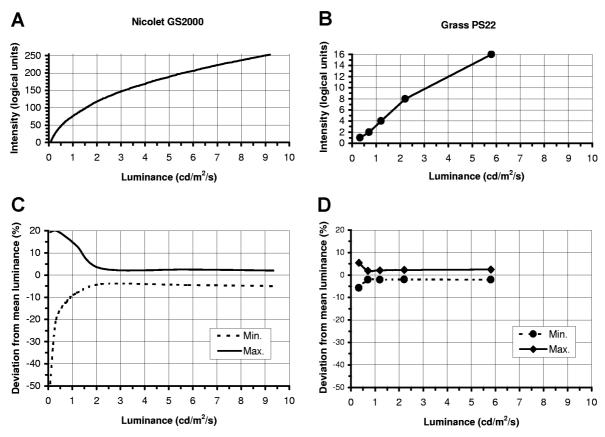
Figure 3. Flash intensity measured at all programmable intesity levels (without filters) of the Nicolet GS2000 stimulator (A) and the Grass PS22 photostimulator (B). Maximal and minimal deviation from the mean intensity in % of the Nicolet (C) and the Grass photostimulator (D).
