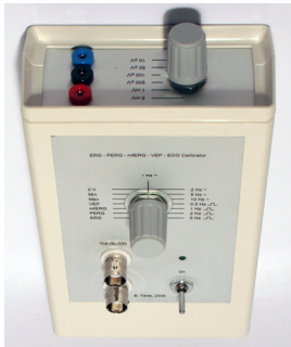
Fig. 1 The Calibrator is a battery-powered microprocessor-controlled signal generator. The operating mode and the output voltage can be selected with the switches on the top and the front side of the unit.
