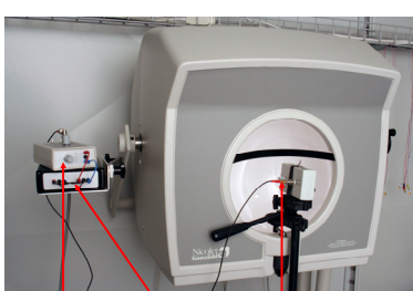
Fig. 2 Calibration of the ERG recording equipment. A light detector triggers the calibration device. The low level signals generated by the calibration device are connected to the inputs of the preamplifier. The sinusoidal transient signal is identified by the recording software as a- and b-Waves. Since voltage and time delay of the generated signals are known (a-Wave 250 µV @ 25 ms and b-Wave 300 µV @ 50 ms), the calibration of the amplification and the calculation of the time shift (4 ms) of the a- and b-Waves can be done without making additional measurements.
